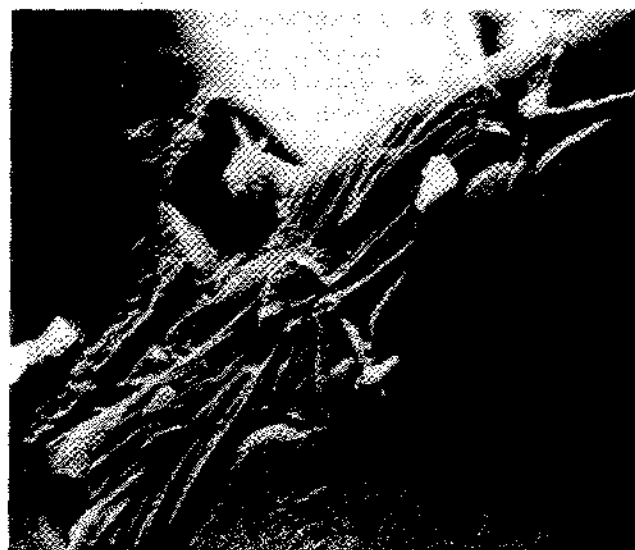
Figure 7. Scanning electron microscope fractography showing polycrystalline inclusion within a cavity closely moulded on it. The rod-shaped crystals are anhydrite, the others contain potassium. (Rock salt from Tersanne, length of the photograph = 91\text{ }\mu\text{m} ).
